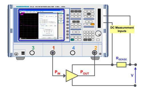
Connection to the DC measurement inputs on the rear of the ZVB can be made with the optional ZV-Z71 cable.
