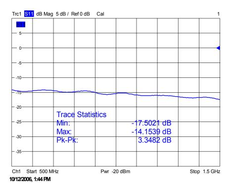
A nice feature of the ZVB is the ability to display the statistical analysis of a desired trace. This can be accessed in the [TRACE FUNCTION] x2 menu and then [Trace Statistics], within this menu you can then choose the required read-out (Min/Max/Peak-Peak etc).
