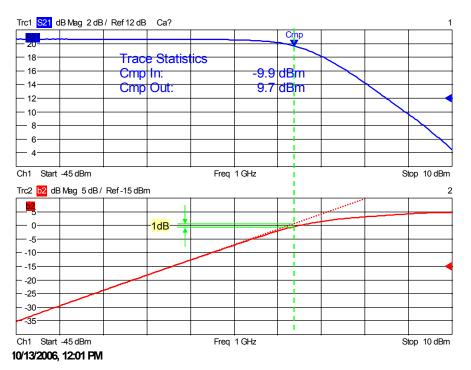
\*Hint, to select more than one compression point value use additional channels with a power sweep at different fixed frequencies.
