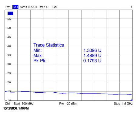
The reflection coefficient can also be displayed in a complex input impedance format that is mapped directly onto the smith chart. This can be accessed using the [Smith] selection within the [FORMAT] menu.
