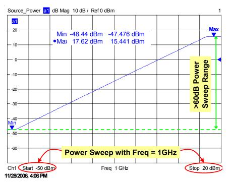
As the S-Parameter  $S_{21}$  is the ratio of the *output power* over *input power*, then this is precisely what is needed to be displayed on the ZVB.
