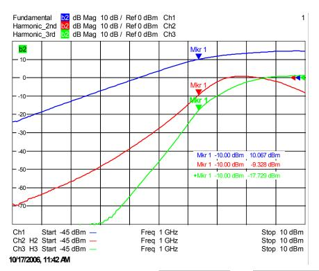
Create a new channel by pressing [CHAN SELECT] and [Add Channel + Trace + Diag Area], and now assign the traces containing the harmonic values to this channel. Select [MODE] and [Harmonics], then choose either 2<sup>nd</sup> Harmonic, 3<sup>rd</sup> Harmonic or another integer multiple of fo from the soft key menu. Multiple harmonic traces can be created by adding a new channel for each, [CHAN SELECT] and [Add Channel + Trace].
