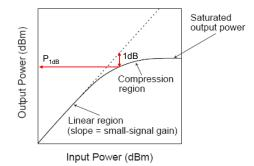
On the ZVB it is possible to not only sweep the measurement versus frequency, but you can also choose power as the swept variable. The ZVB has a very large sweep range available from its generators (typically 60dB), it does this completely electronically without the need for mechanical step attenuators. This makes the ZVB the perfect instrument to measure nonlinearities and compression of an active device.
