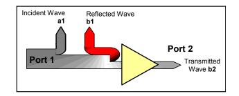
This measured parameter is displayed on the network analyzer as the *S*-*Parameter*,  $S_{11}$  which is the ratio of the *measured power* **b1** divided by the *reference power* **a1**:
