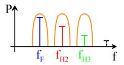
The flexible hardware concept of the ZVB makes it possible to introduce a frequency offset between the generators and the receivers of the instrument (requires ZVB-K3 option). This gives the ability to stimulate the device at the fundamental frequency and then measure the transmission response from the device at a different (multiples of) frequency.
